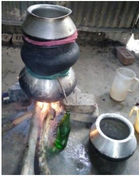
123. Social and cultural tools- Silver pot with shorter neck, mwkhra koro , and bigger silver pot with pipe (Modern method of preparing distilled liquor with pipe)
