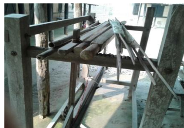
142. Weaving loom, saal- gandwi (wrap and cloth roller), tath (Slay), Gonsha (bamboo stick), Bodangi (bamboo pole), Gorkha (lever), Ban gwja (tool for hanging tath ) and Saal- khuntha (wooden Posts).
