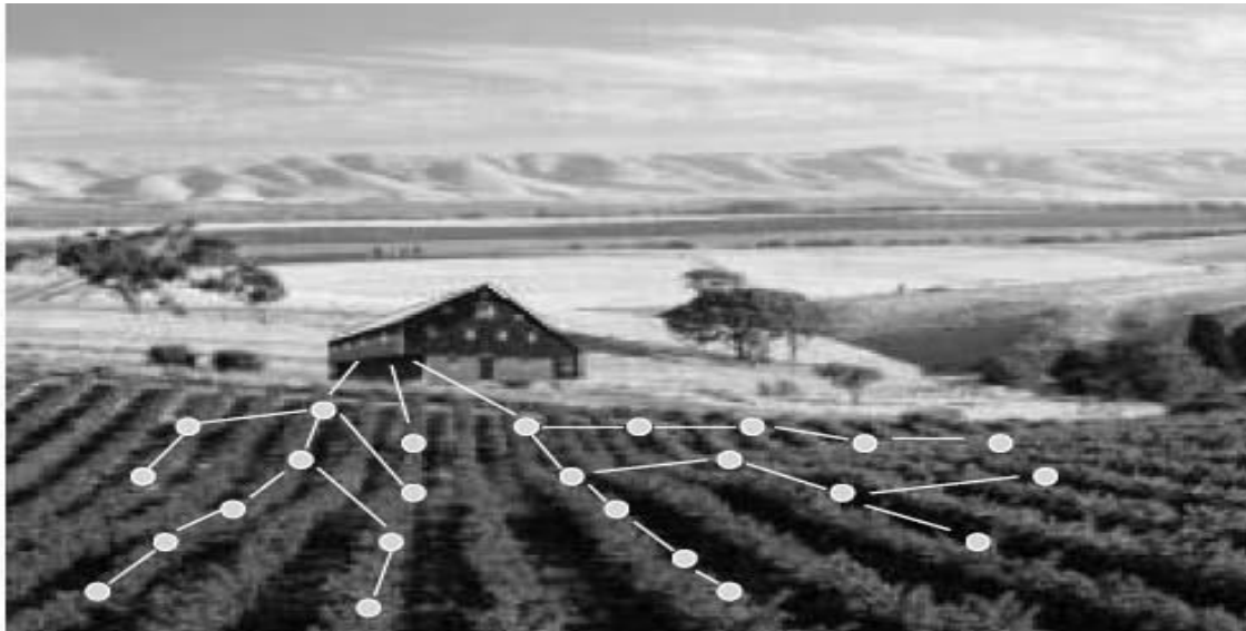
Figure 2.9: Possible deployment Sensors detect temperature, light levels and soil moisture at hundreds of points across a field and communicate their data over a multi-hop network for analysis.
