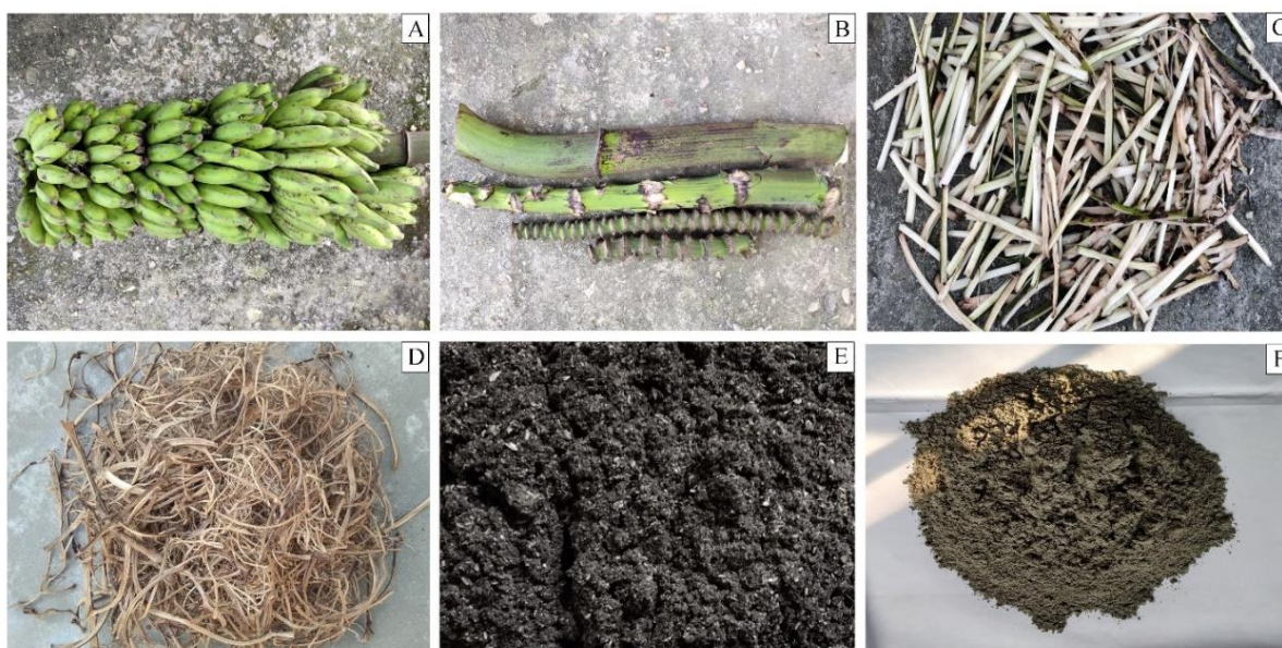
Fig. 3.1. M. champa peduncle (B) obtained from harvesting fruit (A), cut into pieces (C), sun dried (D), burnt ash (E) and calcined catalyst (F).
