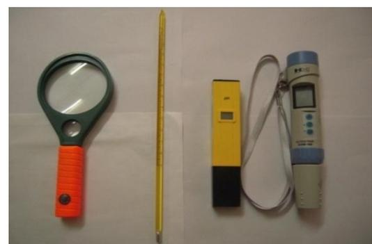
Electronic equipments for EC,Temp, pH, Magnified Glass
