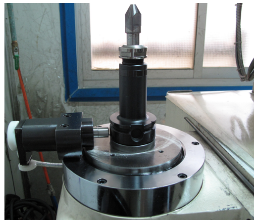
Figure 2: Read/write device on the tool presetter
