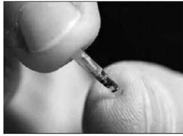
Figure 3.11 Glass transponder for the identification of animals (and humans).
