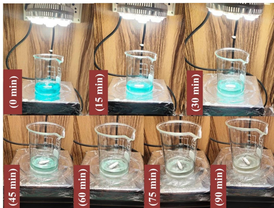
Figure 5.18. Photographic representation of MB degradation, captured at 15-minute intervals during visible-light irradiation of the MB solution containing the ANC photocatalyst, from 0 to 90 minutes.
